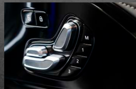
Driver Seat 6-Way Electric Adjustment with Memory Function
